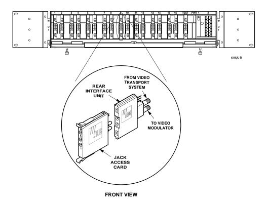
Figure 1. Jack Access Card and Rear Interface Unit
